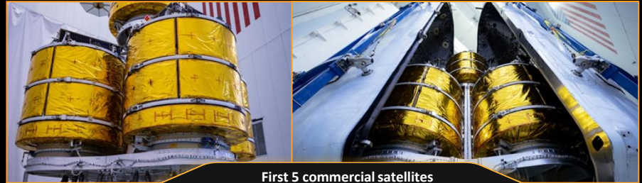
First 5 commercial satellites loaded into the Falcon 9 rocket
