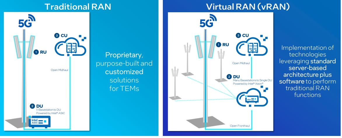
**RU:** Radio Unit **DU:** Distributed Unit **CU:** Centralized Unit
